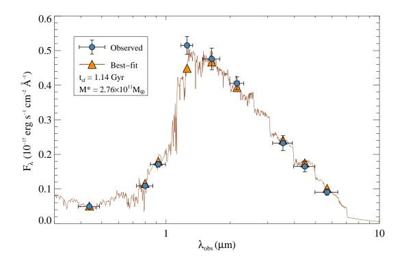
Figure 2. Observed SED for #254025 (blue circles with error bars) compared to the best fit model from Maraston (2005; orange line and symbols). The best fit was found for a SFH with delayed exponential star formation rate that continued for about 1.4 Gyr, with a star-formation timescale of 0.13 Gyr, and for a solar metallicity. The parameters of the best fit templates can be found in Table 1.
