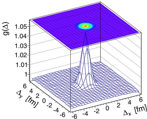
FIG. 5. (Color online) The half-integrated pair correlation function  $g(\Delta)$  for Pb-Pb collisions at impact parameter  $b = 0$  with  $\sigma_{NN}^{\text{inel}} = 20$  mb and  $n = 371$ . No  $NN$  repulsion in the nuclear distributions is included. A sharp peak from the twin-production mechanism is clearly visible.
