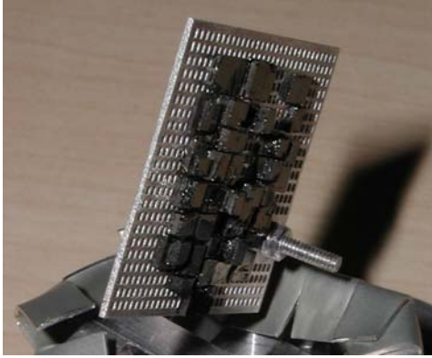
Fig. S1: Photograph of the YBa 2 Cu 3 O 6.45 sample used in this experiment. The Al-plate carrying the crystals is perforated to reduce the amount of Al in the neutron beam, which can give rise to spurious scattering. The c -axis is perpendicular to the plate surface. Up to three crystals are stacked on top of each other (the back side of the plate is similarly covered with crystals). This is to concentrate the sample in the middle of the beam and to avoid the necessity of a second Al-plate.
