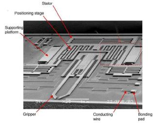
Fig. 6. Single crystal silicon monolithically integrated microgripper, actuated by two linear and one vertical comb actuators [21]. The displacement of the gripper is 5.9  $\mu$ m under a 50 V driving voltage.
