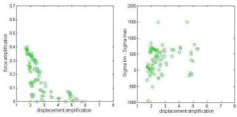
Fig. 12. Pareto front obtained for the optimization with the stress criterion. The structures which have a negative stress criterion are not valid, because  $\sigma_{max} \ge \sigma_{lim}$  (i.e. Von Mises stress greater than yield stress)
