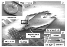
Fig. 1. Articulated polysilicon micro-gripper developed at I.E.M.N. (C.N.R.S.) [51], and actuated by 16 Scratch Drived Actuators.
