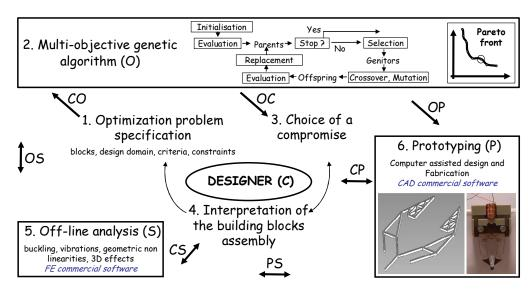
Fig. 9. FlexIn optimal design method of compliant structures: Flowchart of the algorithm (multicriteria optimization).
