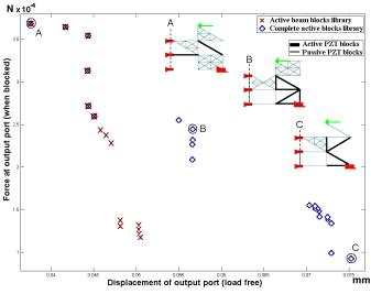
Fig. 14. Pareto graph of piezoelectric compliant microgrippers synthesized using FlexIn (half gripper dimensions are 5 mm  $\times$  9 mm, the thickness is 10  $\mu$ m, PZT material is PIC 151 from PI Piezo Ceramic Technology [57], the input voltage is 150 V). A, B and C are selected half-topologies (markers are boundary conditions, arrow is the output displacement optimized).
