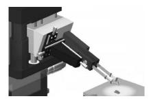
Fig. 3. Flexure hinge micro-gripper, actuated by two piezoelectric bender actuators, for clean environment working [2]. (arms :  $103 \text{ mm} \times 62 \text{ mm} \times 70 \text{ mm}$ ).
