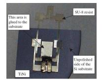
Fig. 4. Compliant SU-8 microgripper actuated by SMA thin film  $(17 \text{ mm} \times 6 \text{ mm} \times 145 \text{ } \mu\text{m})$  [58]
