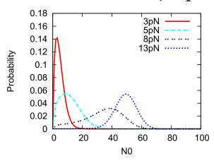
**Figure 4.** Probability distributions of the number of filaments in contact with the barrier at various forces. The parameters are N = 100,  $\gamma = 1$  and  $C = 0.24 \,\mu\text{m}$ .
