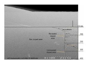
Figure 10: Lateral doping diffusion after thermal annealing
