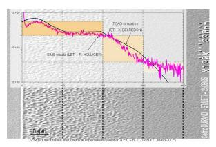
Figure 9: Depth doping level characterization after phosphorous doping
