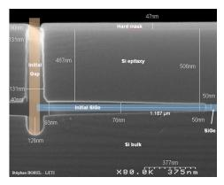
Figure 14: Cross section view of a released tunnel
