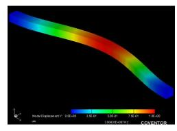
Figure 3: FEM modal simulation of a clamped-clamped beam
