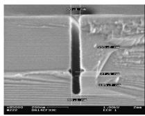
Figure 12: Gap etch cross SEM picture
