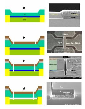
Figure 7: STMicroelectronics SON process
