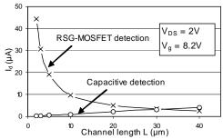
Figure 5: Comparison of MOS & Capacitive detection for a flexural mode clamped-clamped beam
