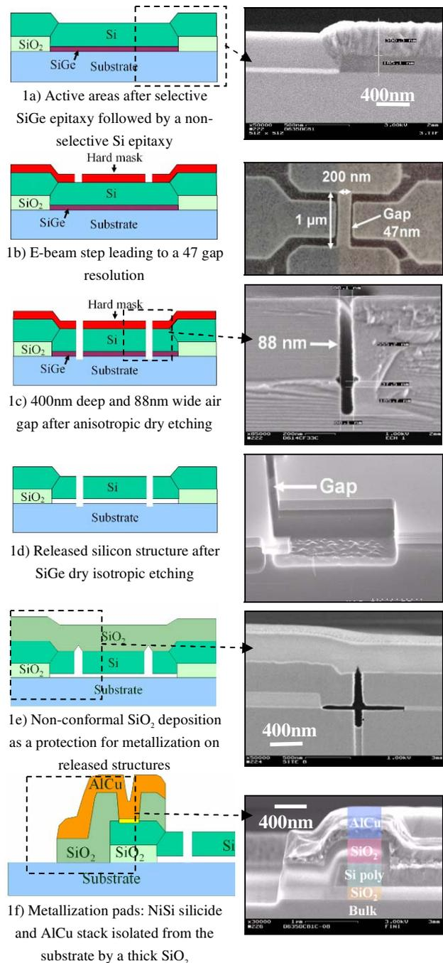
Figure 1: Fabrication process flow and SEM illustrations
