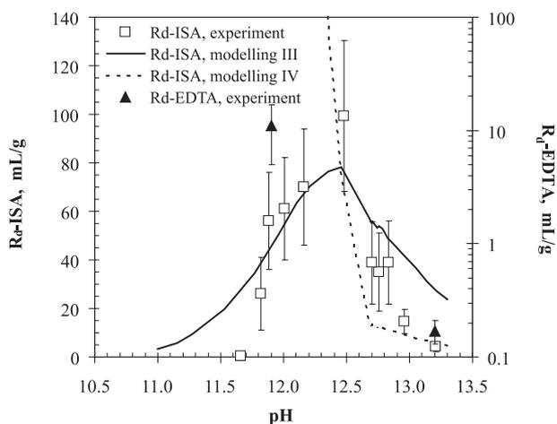
**Fig. 6.** Evolution of the  $R_d$  values of ISA and EDTA in fresh ( $\text{pH} = 13.3$ ) and degraded ( $\text{pH} = 11.9$ ) HCP suspensions. Calculated  $R_d$  values of ISA in HCP suspensions are also represented, using surface equilibria III and IV.
