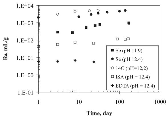
**Fig. 2.** The uptake kinetic of  $^{75}\text{SeO}_3^{2-}$ ,  $^{14}\text{CO}_3^{2-}$ , ISA and EDTA by HCP CEM-I is represented at different degradation states. Kinetic  $R_d$  values of  $^{75}\text{SeO}_3^{2-}$  reported at the degraded state pH 12.4 are issued from [25].
