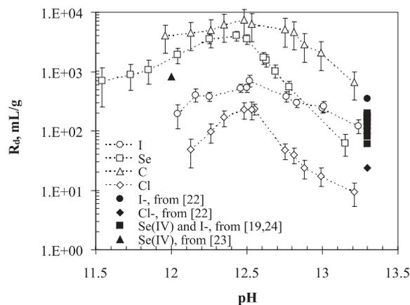
**Fig. 3.** Evolution of the  $R_d$  values of  $^{125}\text{I}^-$ ,  $^{14}\text{CO}_3^{2-}$ ,  $^{75}\text{SeO}_3^{2-}$  and  $^{36}\text{Cl}^-$  in degraded CEM-I HCP suspensions as a function of pH.
