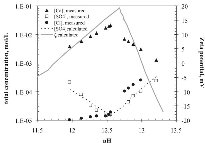
**Fig. 1.** Evolution of the total concentrations of calcium, sulphate and chloride as a function of pH in the suspensions of CEM-I HCP powder in contact with demineralised and decarbonated water and/or artificial fresh cement solution. The error bars of the measured concentrations are contained in the size of the symbols. The evolution of  $[\text{SO}_4^{2-}]$  resulting from the modelling is also reported.  $\zeta$  values are issued from [4].
