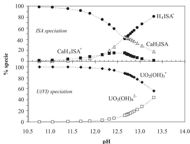
Fig. 5. Speciation of U(VI) and ISA in cement waters as a function of pH and the associated chemical compositions presented in Fig. 1.
