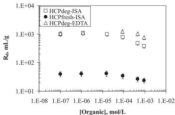
**Fig. 7.** Evolution of the  $R_d$  values of  $^{75}\text{SeO}_3^{2-}$  in fresh ( $\text{pH} = 13.3$ ) and degraded ( $\text{pH} = 11.9$ ) HCP suspensions as a function of ISA or EDTA concentrations. The  $R_d$  values have been measured here after 90 days of contact.
