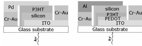
**Fig. 1.** Schematic side-view of the type I (left) and II (right) devices.
