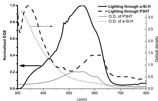
**Fig. 6.** Spectral response (bold) of the device ITO/a-Si:H(n)/a-Si:H(i)/P3HT/Pd when illuminated through silicon (plain) or P3HT (dashed line) and absorption spectra (light) of P3HT (plain) and amorphous silicon (dotted line).
