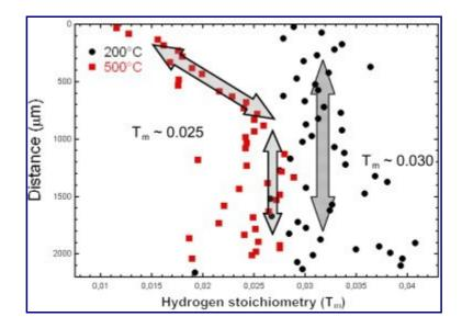
**Fig. 3.** Hydrogen stoichiometry profiles measured on cross sections of ICMCB samples for 20 min annealing at 200 °C (circles) and 500 °C (squares).
