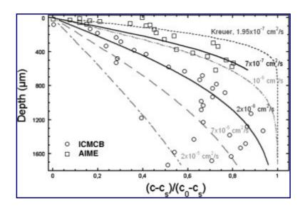
**Fig. 4.** Treated data according to a simple Fickian model and theoretical curves calculated for various diffusion coefficients (squares: AIME, circles: ICMCB).
