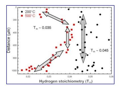
**Fig. 2.** Hydrogen stoichiometry profiles measured on cross sections of AIME samples for 20 min annealing at 200 °C (circles) and 500 °C (squares).
