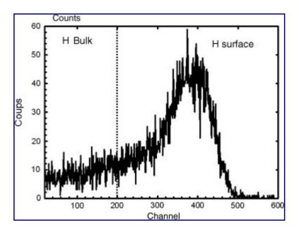
**Fig. 1.** Typical ERDA spectrum measured on BCY10 ceramics. The low energy region of interest is selected to calculate hydrogen concentration.
